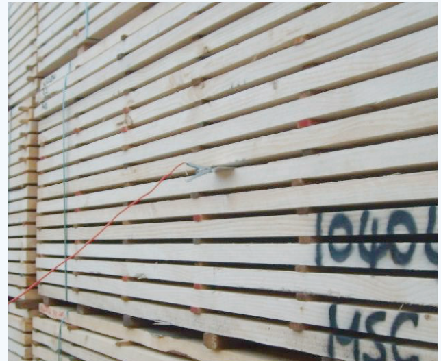
Sensor plates inside the kiln
