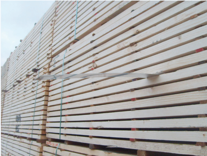
Sensor plates inserted into stack
